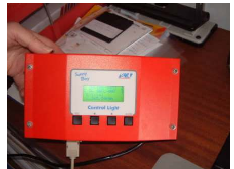
Inverter display panel
